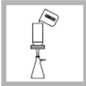
4. Rinse the filter by pouring about 50 mL of deionized water through the filter. Discard the rinse water.
