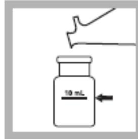
6. **Blank Preparation:** Fill a square sample cell with 10 mL of filtered deionized water from step 5.
